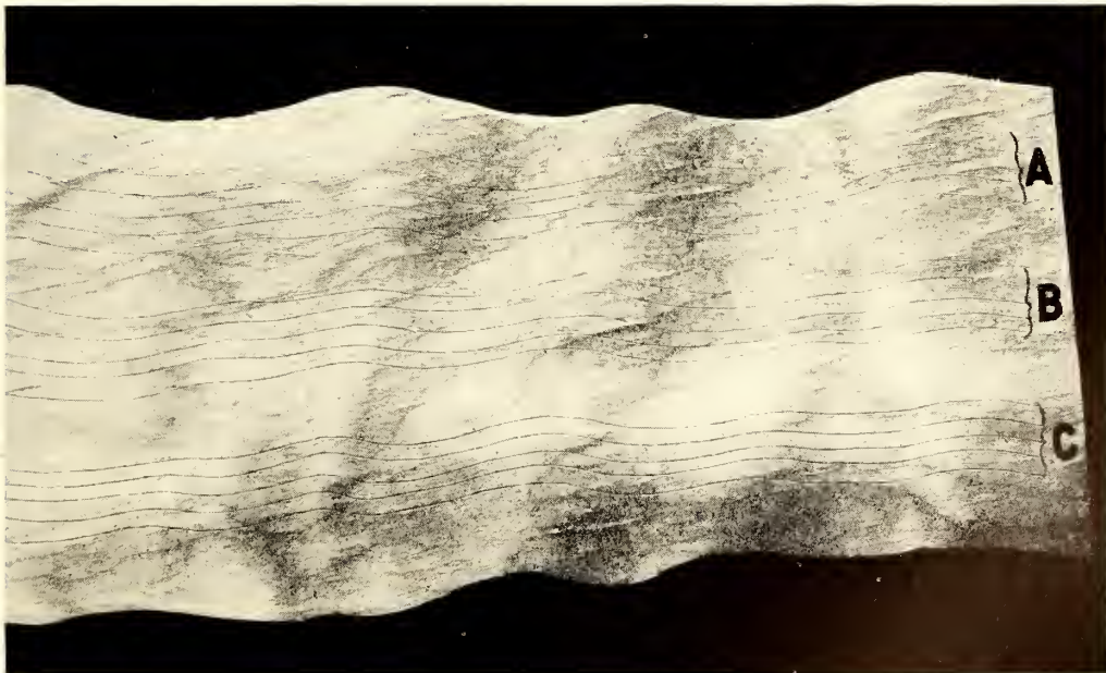
FIGURE 2-56.—Tangential surface of wood tested with scribes to determine direction of grain. Note parallelism of scribe marks in same areas.
